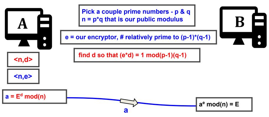
If the E that B calculates in this authentication is the same as it received in encryption phase, then we know the message came from where we thought.
